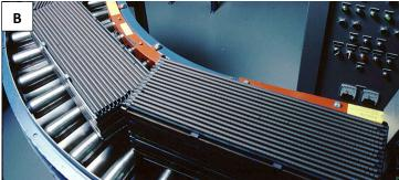
**Figure 4.14:** Fuel fabrication process. A) Uranium dioxide powder compressed into *fuel pellets*. B) Fuel pellets stacked and sealed in metal tubes forming *fuel rods*. C) Fuel rods are bundled into a *fuel assembly*. Images A and B from NRC (public domain); C from RIA Novosti archive, image #132602 / Ruslan Krivobok / CC-BY-SA 3.0
