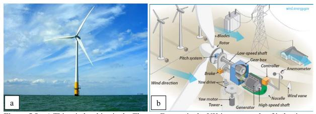
**Figure 5.8. a)** This wind turbine in the Thames Estuary in the UK is an example of induction at work, (credit: Phault, Flickr). Wind pushes the blades of the turbine, spinning a shaft attached to magnets, see image **b** for parts. The magnets spin around a conductive coil, inducing an electric current in the coil, and eventually feeding the electrical grid. Follow this link for an Animation.
