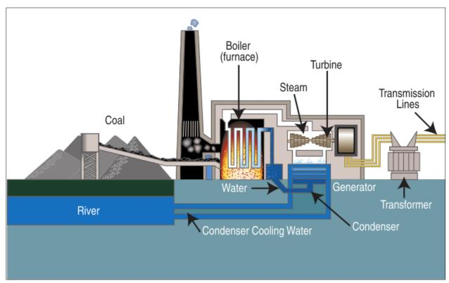
**Figure 4.6:** Diagram of a typical steam-cycle coal power plant (proceeding from left to right). Image by US Tennessee Valley Authority – Public domain. <a href="https://www.tva.com">www.tva.com</a>
