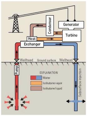
**Figure 5.9**. **a)** Installing a Geothermal Pipe System Drilling to install geothermal ground source pipe system. Source: Office of Sustainability. **b)** Electricity generation at a moderate-temperature hydrothermal system. The geothermal water is used to boil a second fluid (isobutane in this example) whose vapor then drives a turbine generator. The wastewater is injected back into the subsurface. Source: USGS.
