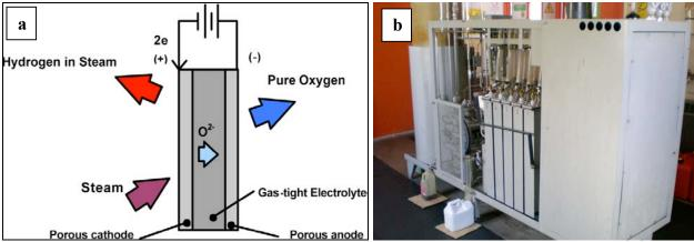
**Figure 5.13 a)** An electric current passed through water resulting in the separation of hydrogen atoms from oxygen to produce the hydrogen fuel. **b)** An electrolyser used in the production of hydrogen by CambridgeBayWeather. After production the hydrogen is used to inflate weather balloons to which a radiosonde is attached. The oxygen produced is vented to the outside.
