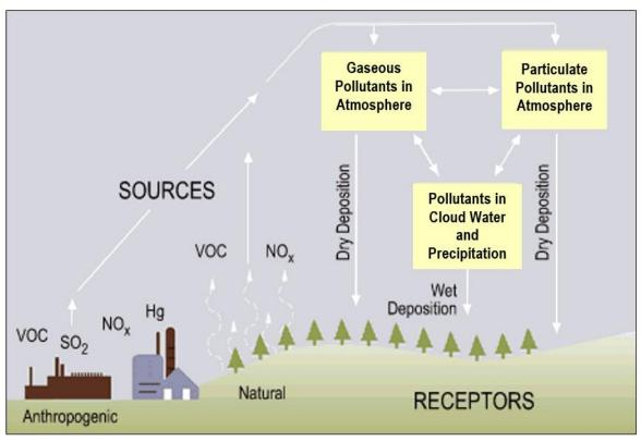
**Figure 6.12**: Formation of acid rain from both natural and anthropogenic pollutants **Source**: US EPA http://www.epa.gov/acidrain/images/origins.gif
