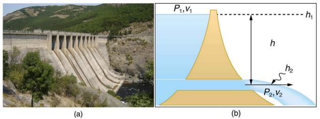
**Figure 5.12.** (a) Water gushes from the base of the Studen Kladenetz dam in Bulgaria. (credit: Kiril Kapustin; http://www.ImagesFromBulgaria.com) (b) In the absence of significant resistance, water flows from the reservoir with the same speed it would have if it fell the distance *h* without friction.
